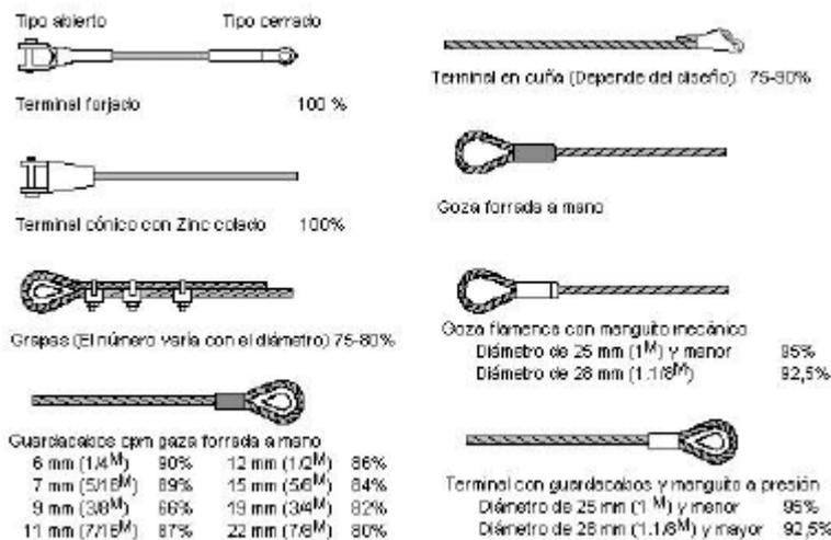
Fig. 8: Load capacity performance depending on end fitting connection
