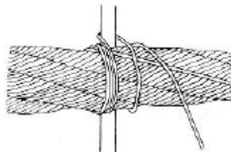
Fig.3: Using a rod to make ties
