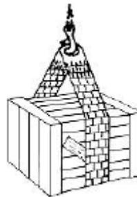
Fig. 7: Band sling (Talurit type)
