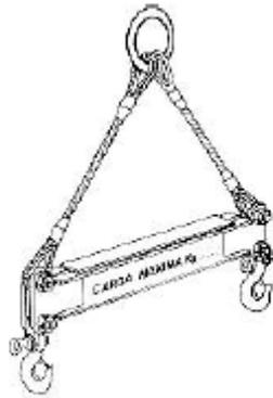
Fig. 11: Portico for lifting loads.
