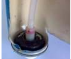
Mounting cup corrosion inside the container
