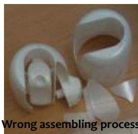
Mounting cups after test Incorrect/correct
